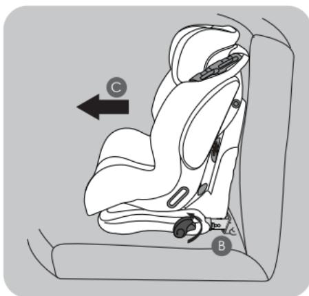
Rotate both adjuster levers (B) anti-clockwise, about a half turn. Do not raise the adjuster levers (B) completely because otherwise, for safety reasons, the stirrups won't extend.
